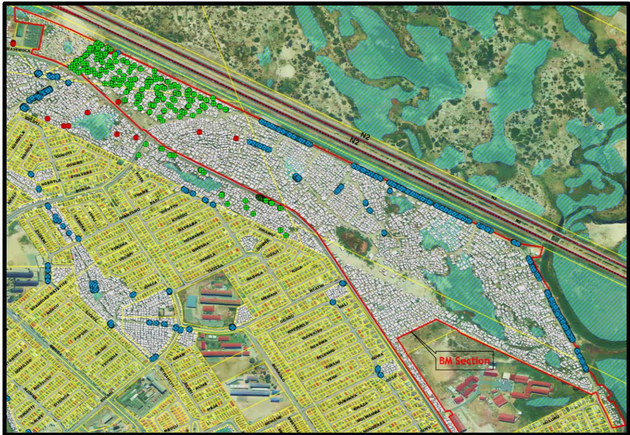
Figure 9: Map of BM Section showing the density and location of full flush shared toilets (Blue), Container toilets (Green), Chemical toilets (Red). Source: City of Cape Town.
